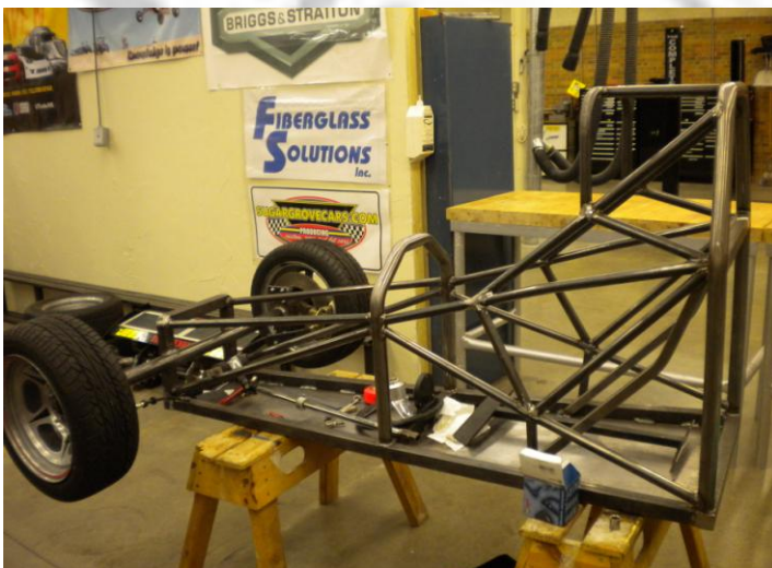
Updated view of the car including floor, front axle, and completed chassis.
